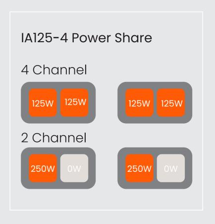
Note: Power Share operates for low impedance 4 & 8 Ohms speakers but channels must be bridged to create a 70V/100V line output.
